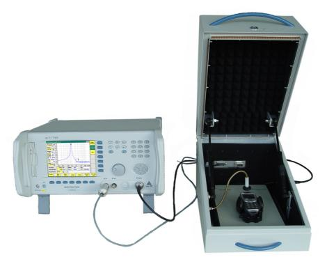
The RF Shield Box Audio Option allows you to perform audio measurements in parallel with radio tests. These measurements lead to consistent Go/NoGo verdicts for the audio parts, based on objective facts rather than personal opinion.
