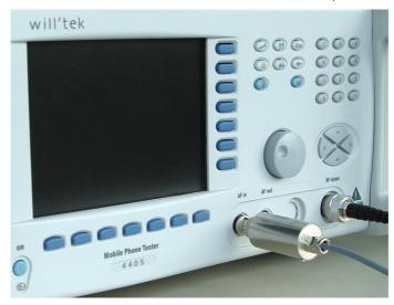
4 When the mobile phone is secured on the Universal Antenna Coupler, place the microphone at its swinging arm over the speaker of the mobile phone, about 1 cm from the phone.
